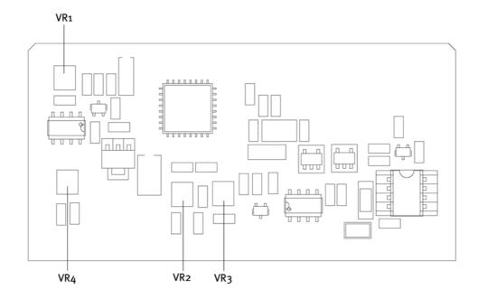
Fig. 21. Internal adjustments positions
